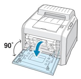
**CAUTION**: If the left cover is not completely open, the top cover release button does not press.
